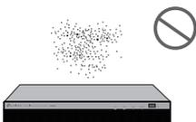
The dust accumulated on the device can be absorbed by static electricity and result in poor contact of metal contact points. Some measures have been taken for the device to prevent static electricity, but too strong static electricity can cause deadly damage to the electronic elements on the internal circuit board. To avoid the effect of static electricity on the operation of the device, attach much importance to the following items:
